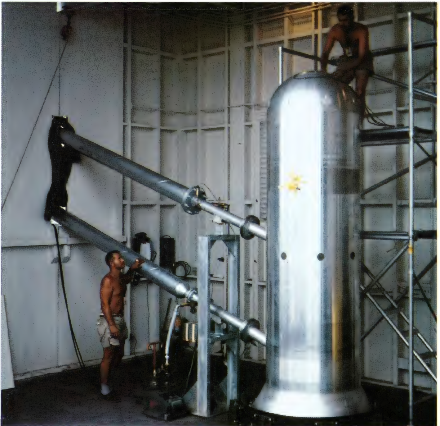
FIGURE 7-33. TEWA DEVICE (D-3, HOB = 8.2' ABOVE WATERLINE)
