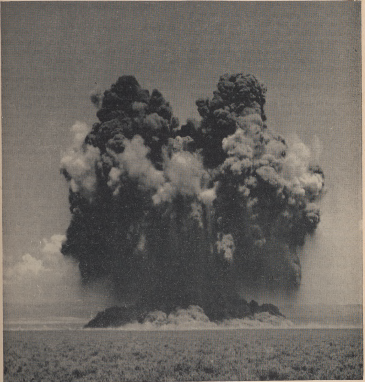
Figure 4.48. Underground explosion of 160 tons of TNT conducted at Dugway Proving Ground, Utah, in May of 1951. The base surge can be clearly seen during the early stages of formation. The similarity of the appearance of this explosion with the underwater atomic explosion shown in fig. 1.25 should be noted.
