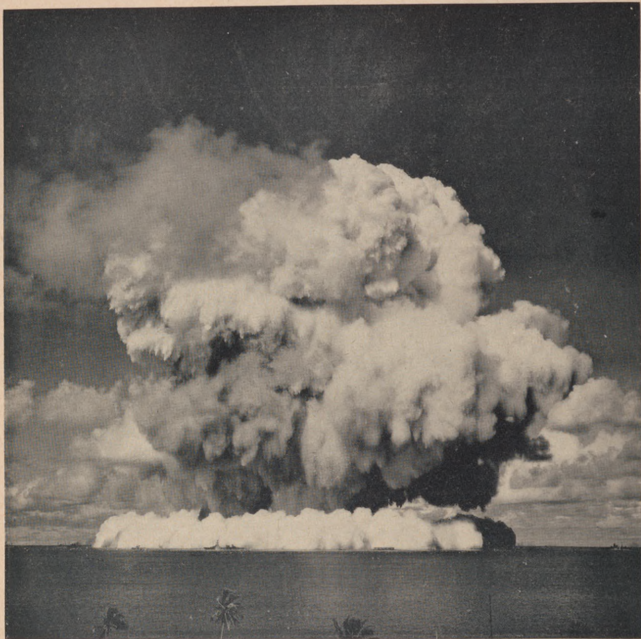
Figure 1.25. Initial stage of the base surge at the base of the water column in Test Baker.
