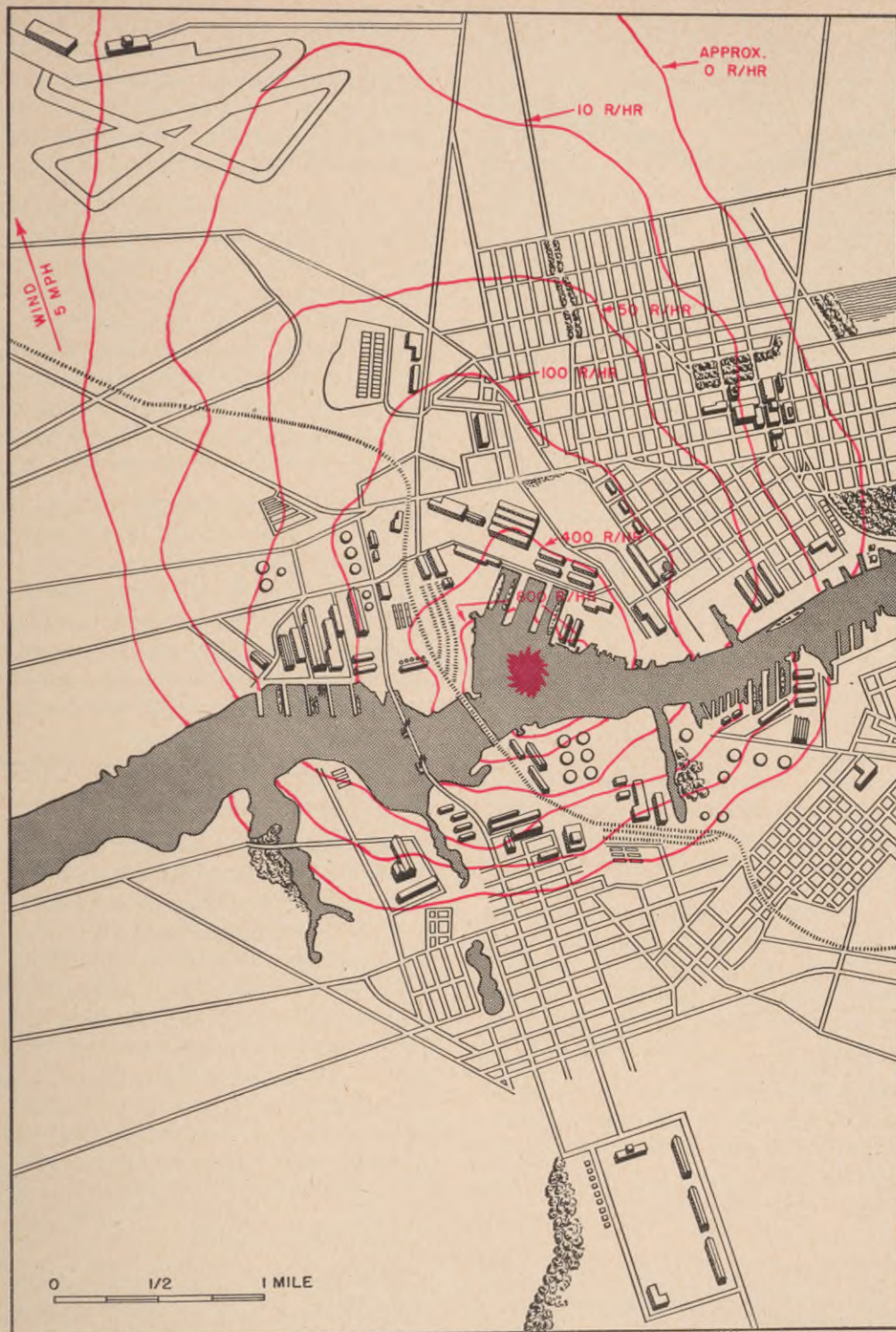
Figure 9.30b. Map of a typical municipal and harbor area. Dose-rate contours show monitoring data corrected to one hour after detonation as in figure 9.30a, except that an underwater burst with 5 m.p.h. wind was assumed.
