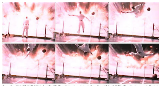
Operation SAILOR HAT, 0.5 kt shot CHARLIE, at Kahoolawe Island, Hawaii, on 16 April 1955. The displacement effects to a standing observer at a peak overpressure of 8 psi (41 kPa) were simulated by using a realistic (fully articulated) dummy.
