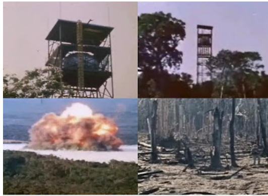
Operation BLOWDOWN: an Australian-British-American 0.05 kt test on a 43 m high tower in a rainforest at Iron Range, Northern Queensland, on 18 July 1963 to assess the dynamic pressures required for tree blowdown, and the difficulty in moving through the blowdown area.
