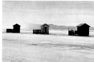
Figure 7.57. Wooden test houses before exposure to a nuclear explosion, Nevada Test Site.
