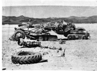
Figure 12.4b: Earth-moving equipment subjected to nuclear blast in open terrain (30 psi overpressure).
